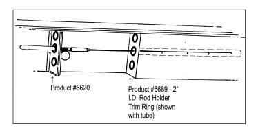
6698 - Rod Holder Trim Rings and Tubes are typically used for horizontal rod storage while underway. Prior to drilling holes, make certain you have adequate space for the tubes that serve to protect your rods.
