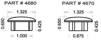
Drill 1" or 7/8" hole, position cap, and drive in with soft mallet.
