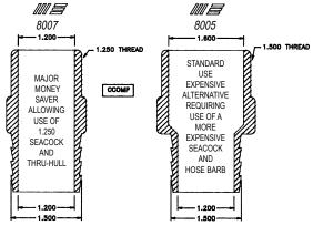
THE FLOW OF LIQUIDS THROUGH THESE TWO PARTS ARE IDENTICAL AS IT IS GOVERNED BY THE 1.200 INCH DIAMETER OF THE BARB
