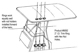
6695 - The above drawing shows a typical thru-the-top installation. Rod holders and/ or supports are installed through the canvas or fiberglass top directly above your boat's console-mounted rod holders.
