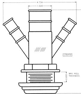
Marine East new TRIPLE THRU HULL allows three outlets through a single thru hull opening. Increasing safety while simplifying installation.
