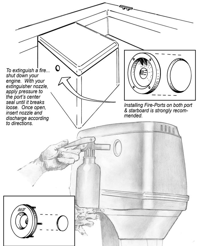
To extinguish a fire... shut down your engine. With your extinguisher nozzle, apply pressure to the port's center seal until it breaks loose. Once open, insert nozzle and discharge according to directions.
