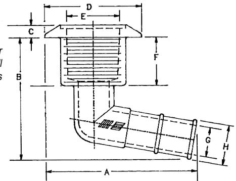
Mushroom head used for all above water thru-hull connections
